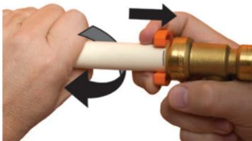
1. Place the SharkBite® disconnect clip around the tube with the non-branded face against the release collar. If using the SharkBite® disconnect tongs, place the teeth around the fitting assembly. The fork end with the SharkBite® brand logo should be positioned around the tube and the other end around the neck of the fitting.
