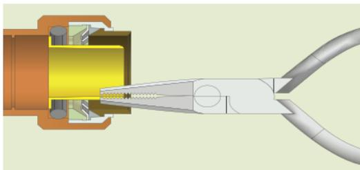
Gently work the Tube Support Liner past the o-ring
