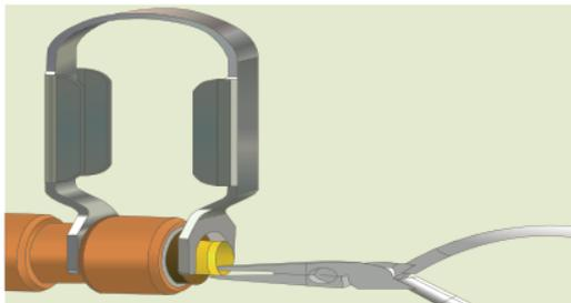
Put the disconnect tongs (or clip) in place and squeeze them together. This will cause the grab ring teeth to spread.
