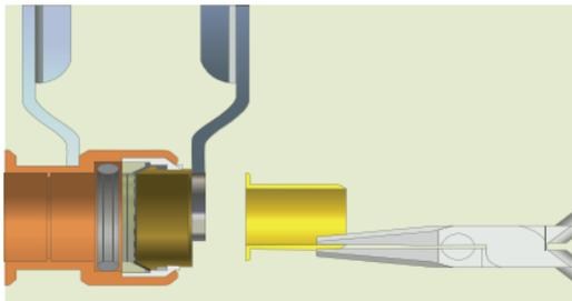
Once the disconnect tongs are squeezed and the grab ring teeth are spread, the Tube Support Liner can be easily removed.
