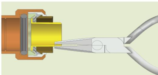
Stop once the Tube Support Liner has been pulled past the o-ring, the Tube Support Liner cannot be pulled out any further due to the grab ring.
